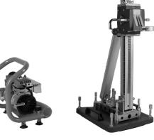
Now switch the vacuum pump to "ON" and wait until a vacuum of 0.9bar is reached. Check the firm hold of the plate and the drill stand.
